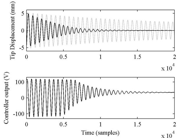
Fig. 3. Uncontrolled (grey) and NRMPC controlled (black) beam tip deflection, caused by an initial deflection of 5mm.
