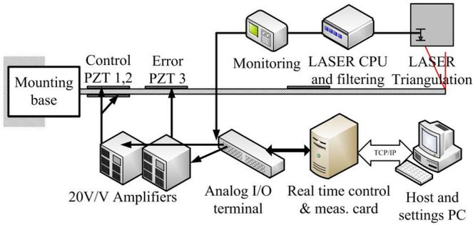
Fig. 1. Experimental device setup scheme.
