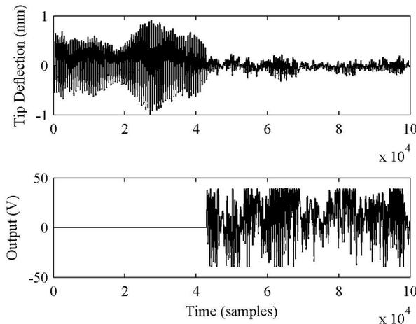
Fig. 5. Uncontrolled and NRMPC controlled beam tip vibration with controller response to a quasi-random excitation.
