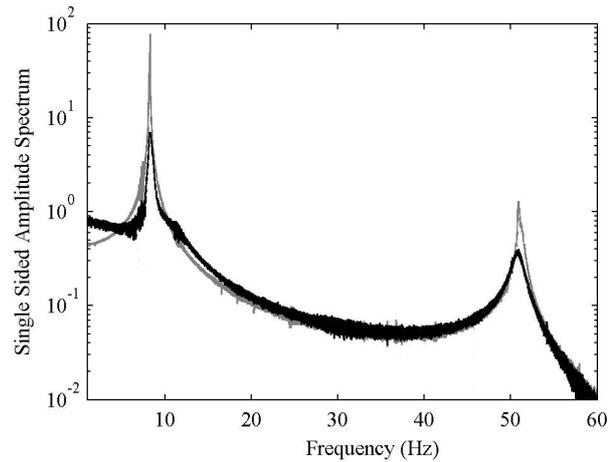
Fig. 4. Uncontrolled (grey) and NRMPC controlled (black) single sided logarithmic amplitude spectrum of the beam tip displacement as a response to a chirp signal.
