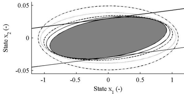
Fig. 2. Projection size with increasing prediction horizon and fixed shift matrix. The innermost ellipse drawn with a solid line denotes  $n_c = 2$  steps the dash-dot outer  $n_c = 32$  steps ahead prediction.
