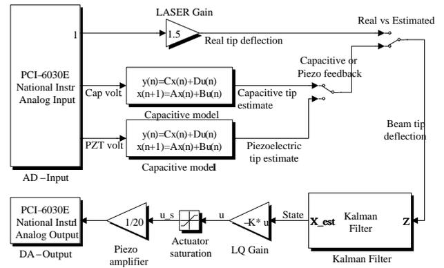
Figure 3. Simplified block scheme of the controller algorithm.
