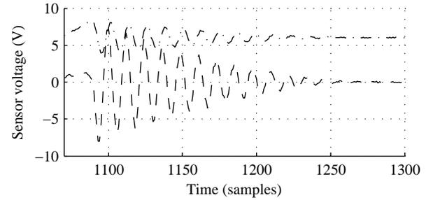
(b) Capacitive and piezoelectric sensor voltages.
