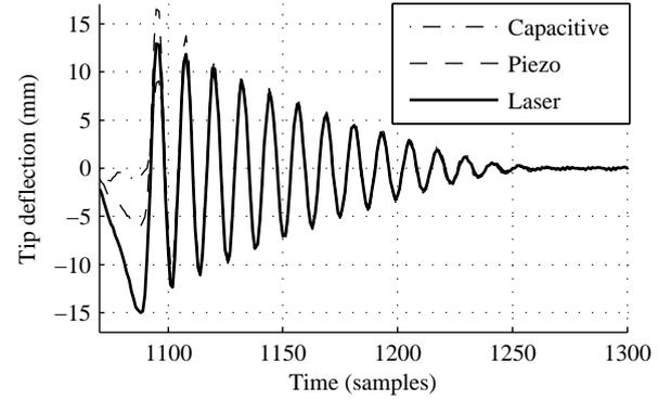
(a) Measured and model estimated beam tip deflection.
