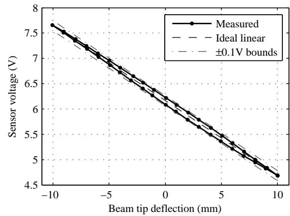
Figure 4. Static characteristics of the capacitive feedback setup, related to beam tip deflection. Dashed line denotes the ideal linear relation, while the solid line indicates actual measurements.
