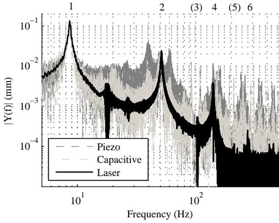
Figure 6. Single-sided amplitude spectrum of measured and estimated beam tip deflections. Numbers denote laser measured amplitude peaks due to corresponding structural vibration modes.
